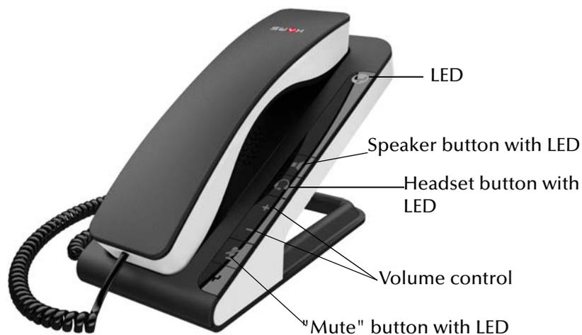
Use the "Plus" and "Minus" buttons to control the volume. Volume control affects the output source (headset, handset, and speakers) currently in use. The "Mute" button activates/deactivates the microphone currently in use. The "Headset" button enables headset mode. The "Speaker" button activates the device speaker.
